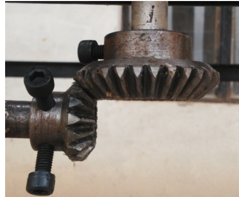
Figure 4. Bevel gears
