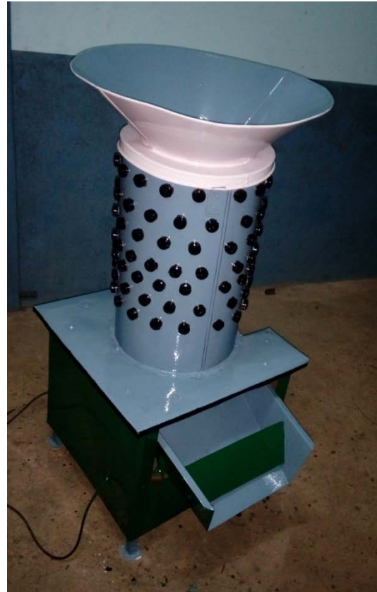
Figure 4. Fabricated Pepper Threshing machine
