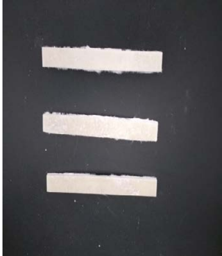
Figure 4. Fabricated flexural specimen
