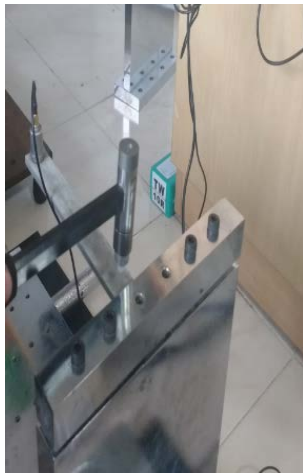
Figure 5. Experimental Setup for vibration test
