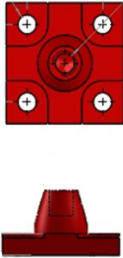
Figure 8. Isolator Configuration –2- Square type
