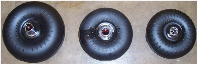
Figure 6. Geometrically scaled torque converters tested with U = 140 , from left to right, 300 mm, 258 mm and 245 mm pump diameters
