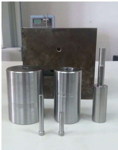
Figure 3. Two-stage extrusion die, punch and die block
