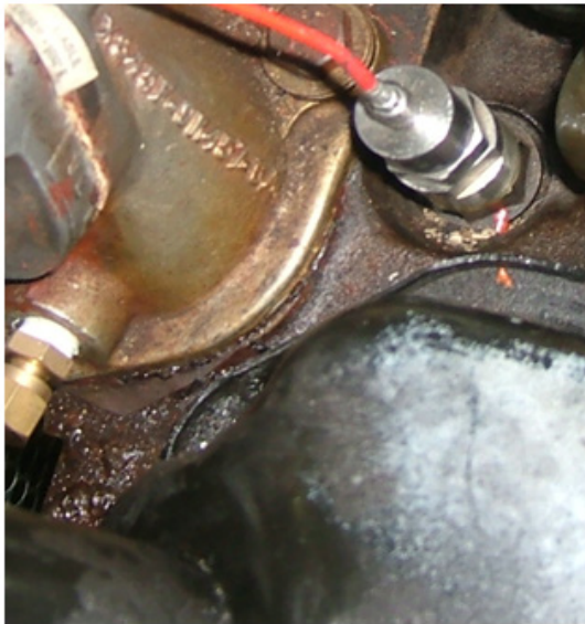
Figure 3. Vibration accelerator type 4368 location
