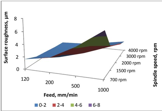
**Figure 4a.** Effect of spindle speed on surface roughness at constant DOC of 0.4mm (dry)
