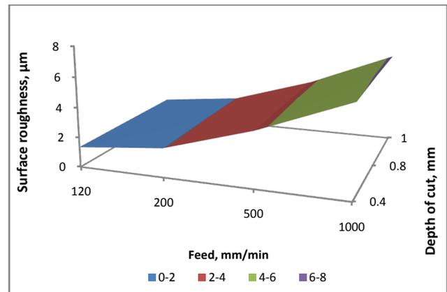
Figure 10b. Effect of DOC on surface at constant spindle speed of 700rpm (MQL)
