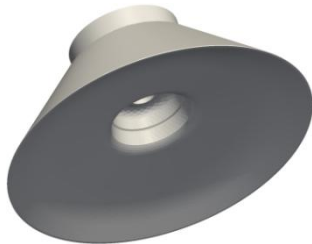
Figure 2. Bell geometry. The bell rotates around its axis and paint is transferred from the center to the edge by the centrifugal force
