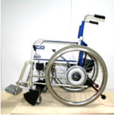
Figure 19. Wheelchair with the Assistive caster units
