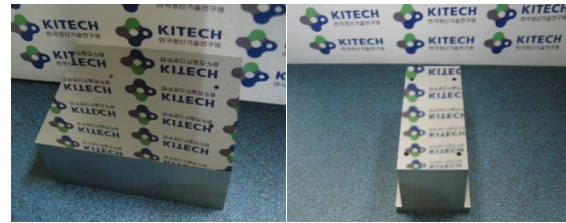
(a) Up and bottom plates after mirror-finishing
