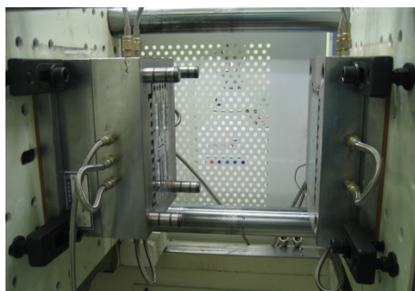
(a) Mold set-up for the test injection
