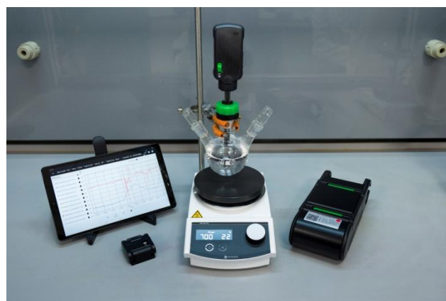
Figure 2. An image of a typical DigitalGlassware® equipment set up in the laboratory. The DeviceX multi-sensor probe is inserted into the reaction flask, on the right the DigitalGlassware® WebApp is running on a tablet. Right front – DeviceX Environmental Sensor that is mounted within the fumehood. Left – Digital Controller
