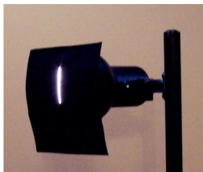
Figure 9. When observing spectrum of a light bulb, one can place a slit on the object itself
