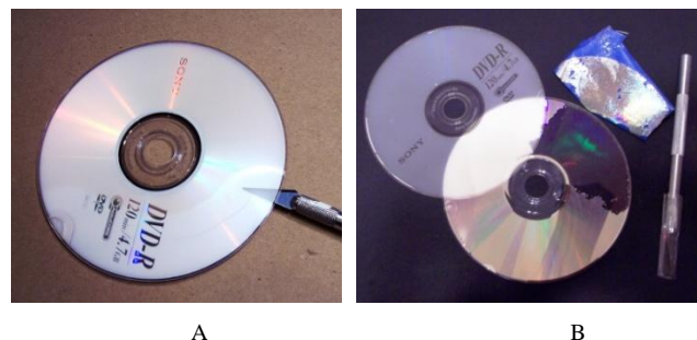
Figure 2. Preparation of a DVD spectroscope. A. Insert a utility knife between the two polycarbonate sheets and force them apart. B. Use an adhesive tape to lift the foil off
