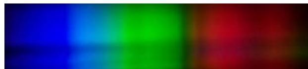
Figure 11. Spectrum of GE Reveal 60 lightbulb. Note absorption bands in the yellow part of the spectrum
