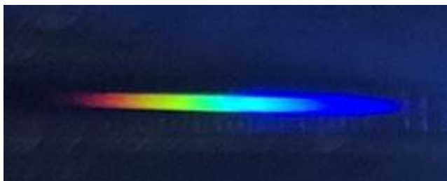
Figure 2. Photo of the 3D spectrometer signal from a 1.0 cm 2 cell filled with water. The light source is a white LED
