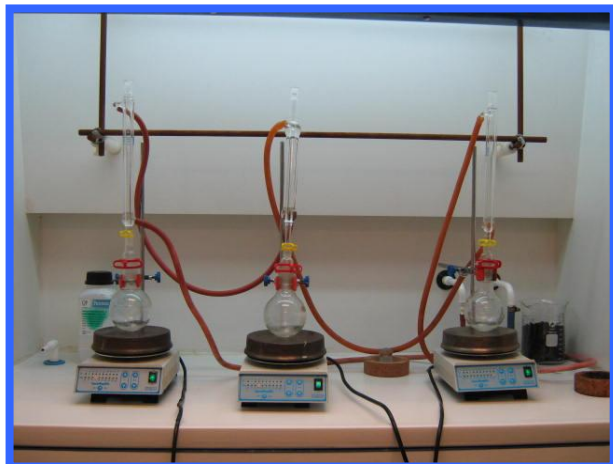
Figure 1. Reflux assembly for the reaction of hydrolysis
