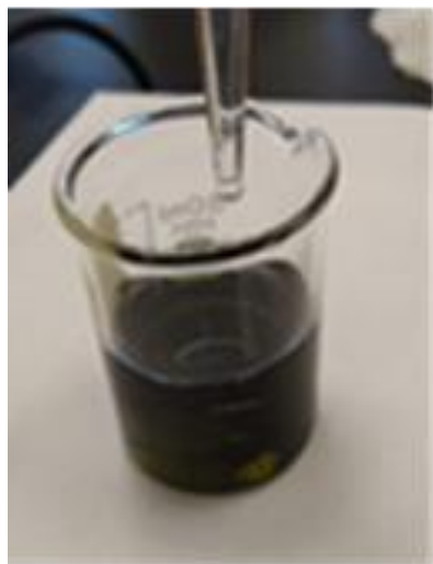
Figure 4. Color of titrated 2,4-DNPacOH solution beyond the end point
