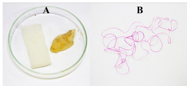
Figure 6. Appearance of polycotton after treatment with pure DMSO (left, no visible change) and BuMeImAcO (right, yellowish material), part A. The regenerated, dyed cellulose fiber from polycotton, part B
