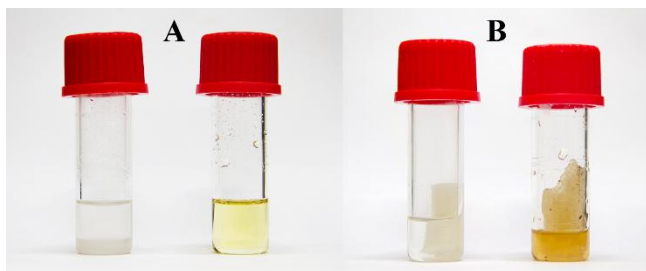
Figure 4. Glass tubes after dissolution procedures with MCC (Part A) and polycotton (Part B). In parts A and B, the tubes to the left refer to pure DMSO (no visible change), whereas those to the right refer to BuMeImAcO-DMSO, yellowish viscous solutions due to cellulose dissolution
