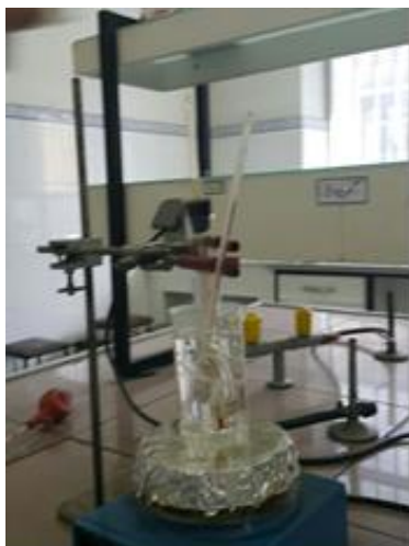
Figure 1. Water bath plus bulky tube containing oleic acid and palmitic acid
