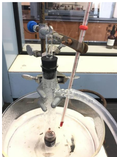
Figure 3. A Pasteur pipet was inserted through a rubber stopper with a drill hole, to serve as air inlet
