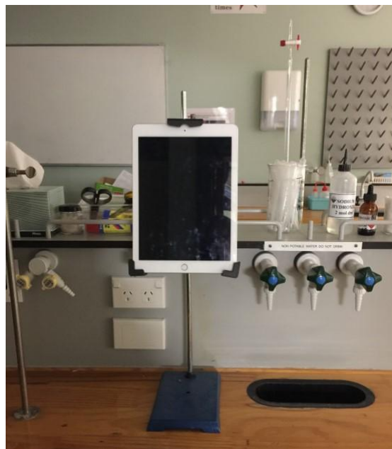
Figure 1. A view of the iPads showing their placement on a retort stand above the laboratory bench
