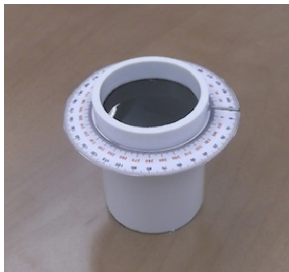
Figure 5. Complete assembly of final polarimeter
