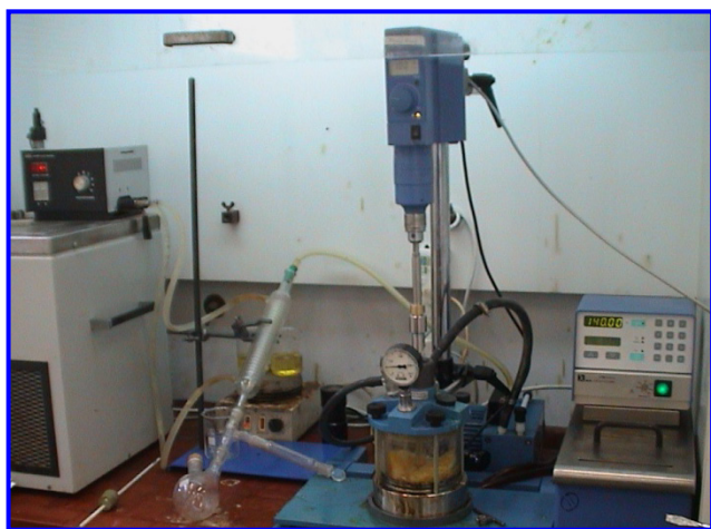
Figure 1. Experimental setup of the polyamidation reaction
