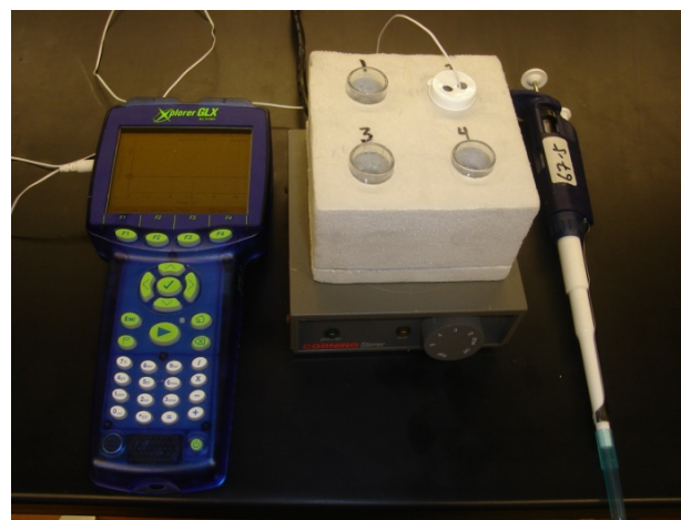
Figure 1. Setup for micro-calorimetry
