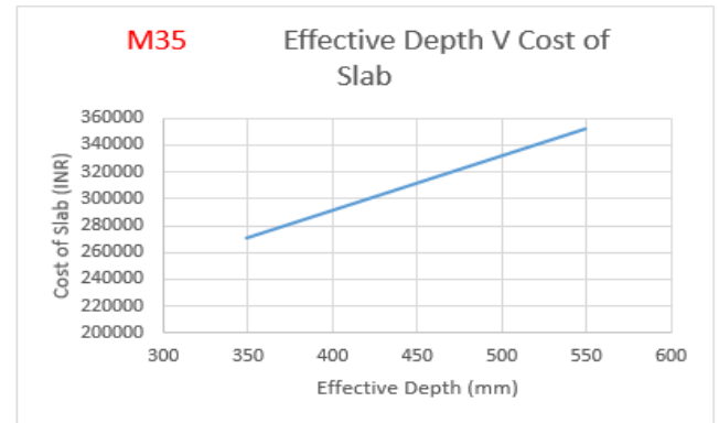
Figure 5(b). Variation of effective depth to cost of slab for M35 Grade Concrete
