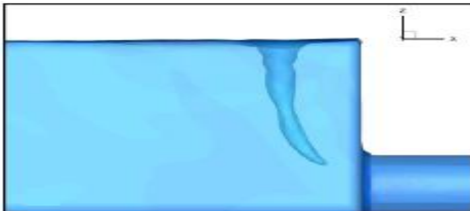
Figure 4. Vortex formation and Critical submergence with coarse mesh
