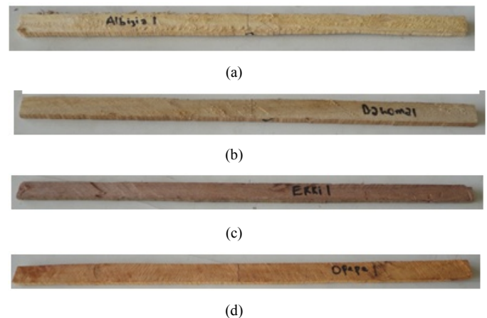
Figure 5. Static bending test specimen shapes and sizes (a) Albizia (b) Ekimi (c) Ekki (d) Opepe
