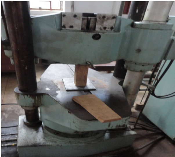
Figure 3. Arrangement of sample for compression test
