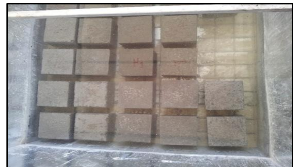
Figure 2. Curing of the concrete specimens
