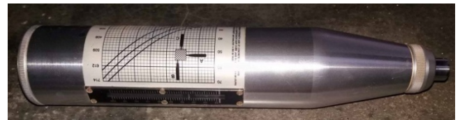
Figure 1. N-type rebound hammer
