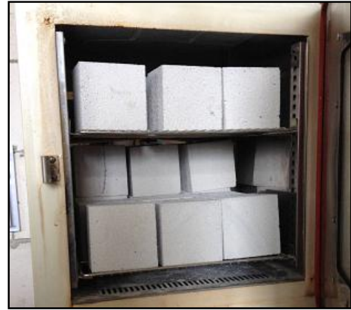
Figure 3. AAC brick samples after autoclaving process in Autoclave
