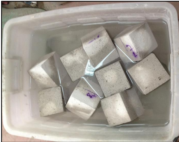
Figure 8. Water absorption test carried out according to TCVN 248:1986
