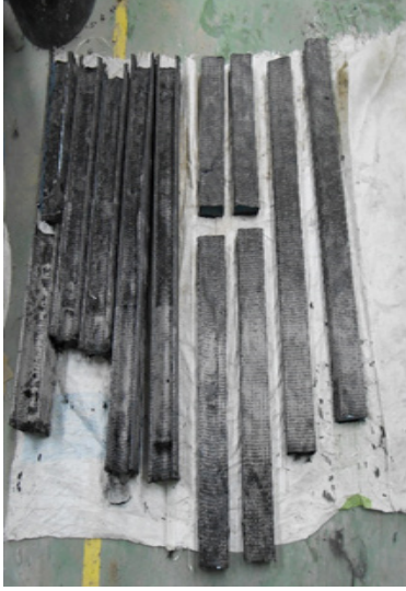
Figure 1. CFRP strengthened specimens
