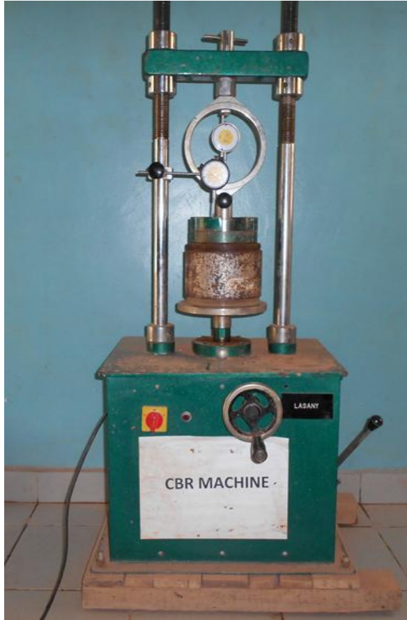
Figure 4. CBR machine set-up
