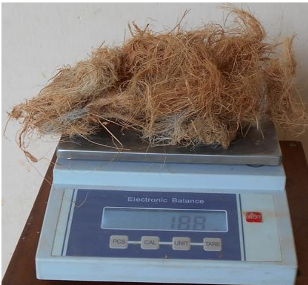
Figure 2. Weighing the fiber to be compacted with the soil
