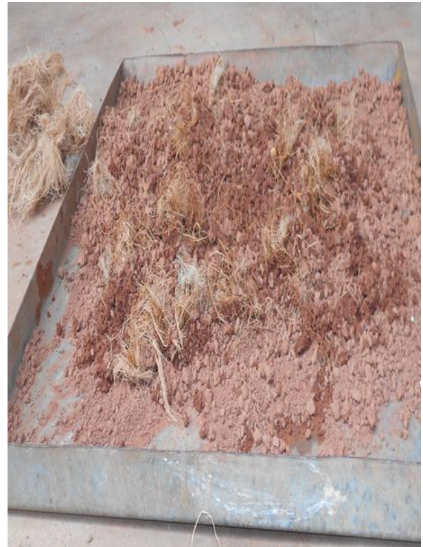
Figure 3. Properly mixing the fiber-soil with water
