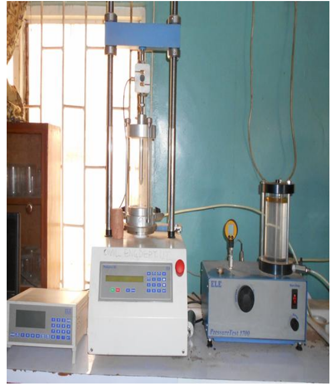
Figure 5. Multiplex 50 set up for shear strength test
