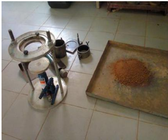
Figure 5. Compaction test set up
