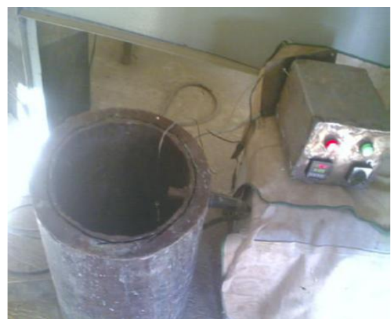
Figure 3. Electric furnace for burning the sludge to whitish powder
