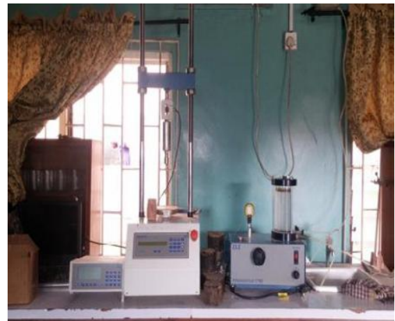
Figure 6. Multiplex 50 set up for shear strength test
