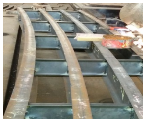
a- Welding Diaphragms
