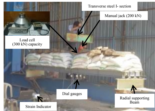
Plate 2. Test Rig Elements
