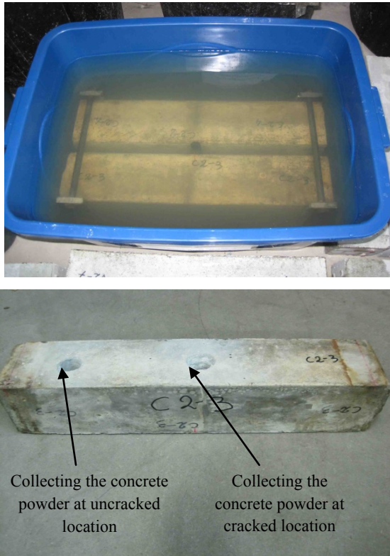
Figure 10. Immersion of cracked beam into salt solution and location for collecting the concrete powder
