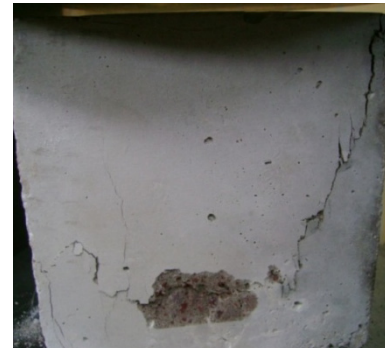
Figure 1. Cube specimen under load
