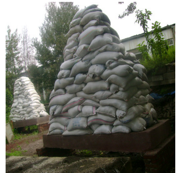
Figure 7b. Ribbed-Slabs 2 and 3 under load
