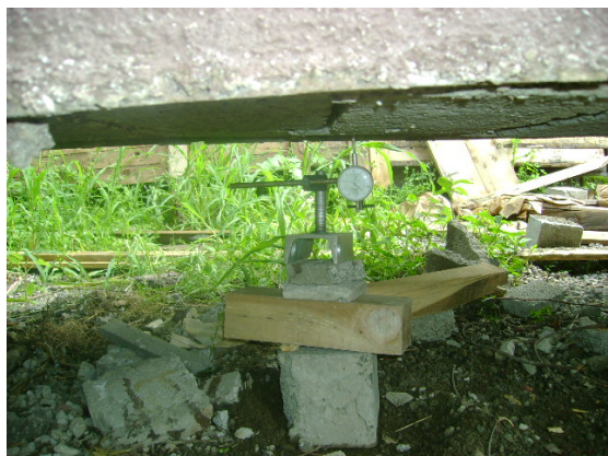
Figure 6. Ribbed-Slab, experimental setup with gauges
