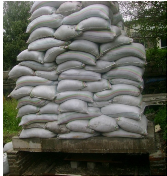
Figure 7a. Ribbed-Slab1 under load
