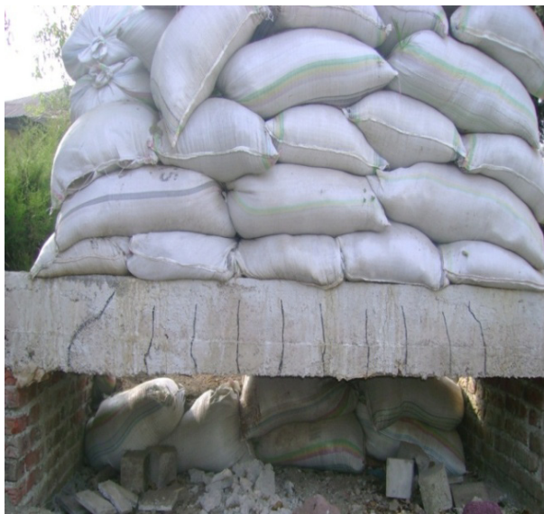
Figure 11. Crack pattern in experiment slab 1
