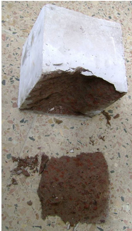
Figure 3. Scoria Aggregates Crushing
