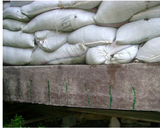
Figure 12. Crack pattern in experiment slab 2
