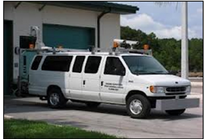
Figure 1. Specialized Van for IRI Data Collection
