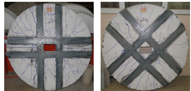
Figure 14. Cracks Pattern for Circular Slabs with Rectangular Openings
