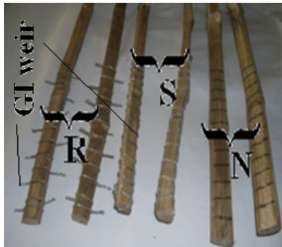
Figure 1. Prepared samples for Pull-out test
