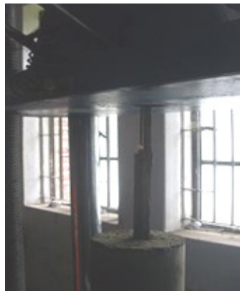
Figure 10. Pull-out test of bamboo
