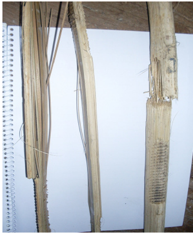
Figure 2. Failed bamboo after Tension test in UTM
