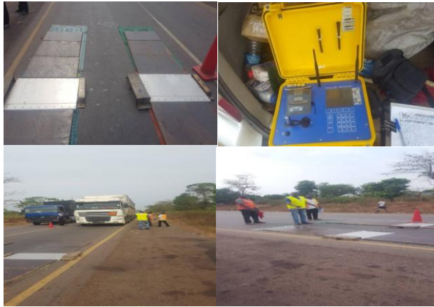
Figure 1. A portable Axle Weigh pad
