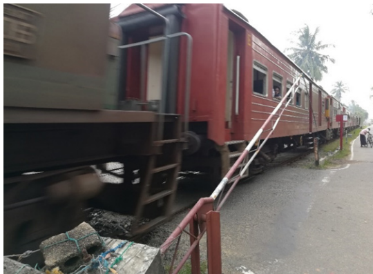
Figure 6. Partially Closed GI Gate
