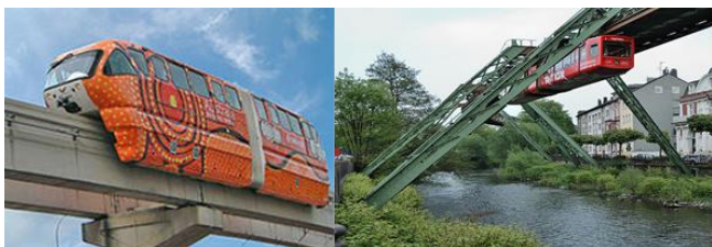
Figure 1. Classic monorail and underslung monorail
