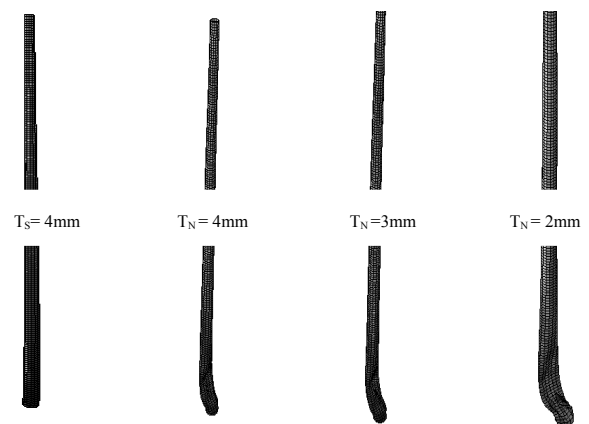
Figure 3. Deformation of the lighting column with different shell thicknesses
