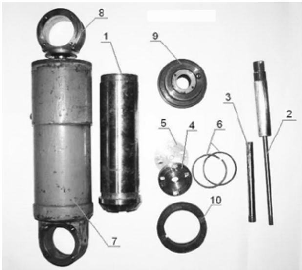
Figure 2. The model sample of a hydromechanical damper
