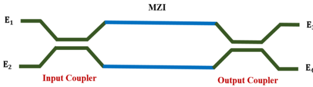
Figure 6. Schematic of the 2 \times 2 Mach-Zehnder switch used in the proposed photonic delay line
