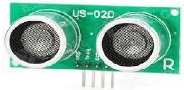
Figure 11. Physical representation of ultrasonic sensor
