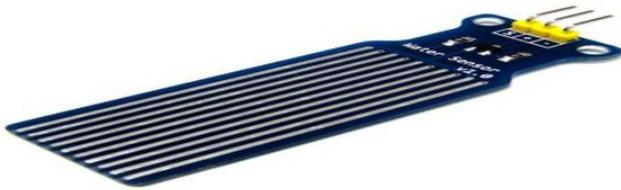
Figure 9. Physical representation of water sensor
