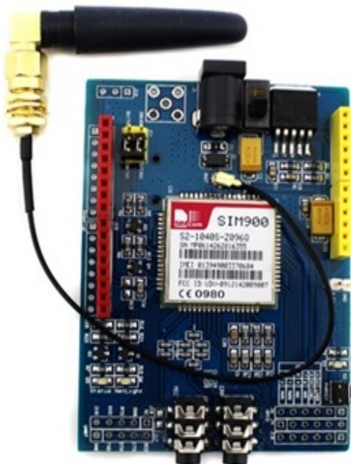
**Figure 7.** SIM900 for Arduino controller
