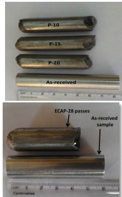
Figure 1. Low carbon steel billet (a) as-received, after ECAP for ten passes (P-10), fifteen passes (P-15), twenty passes (P-20) and (b) twenty eight 28 passes
