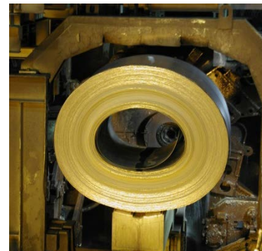
Figure 8. An example of asymmetric contraction of hot coil after coiling[4]
