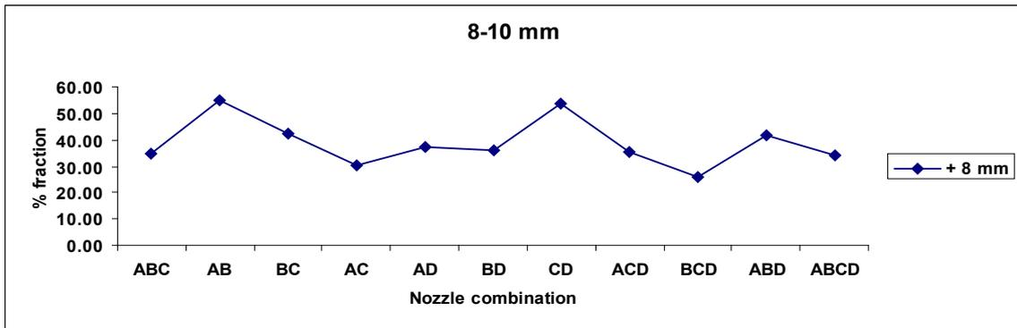
Figure 12. Fraction of 8-10 mm green pellet vs nozzle combination
