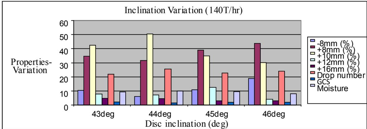
Figure 25. Properties variation vs. disc inclination at feed-rate of 140tph
