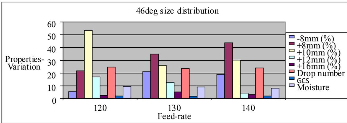
**Figure 22.** Properties variation vs. feed-rate (tph) at 46° of disc inclination
