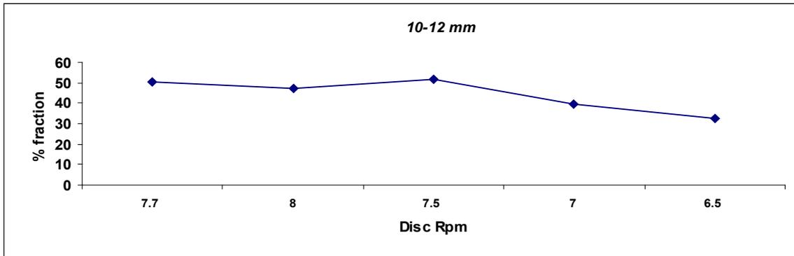
Figure 5. Fraction of 10-12mm size of green pellet vs Disc rpm
