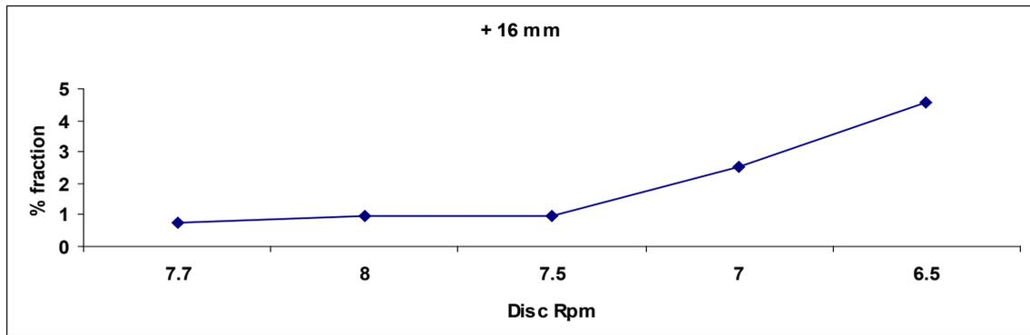
Figure 7. Fraction of +16mm size of green pellet vs Disc rpm
