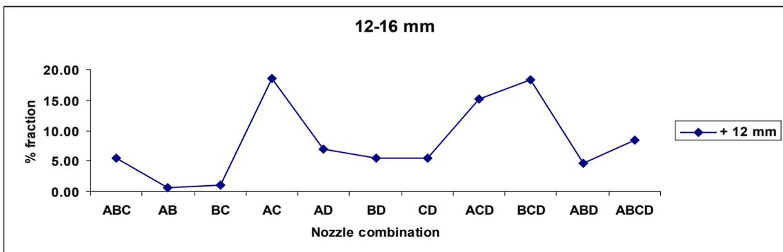
Figure 14. Fraction of 12-16 mm green pellet vs nozzle combination
