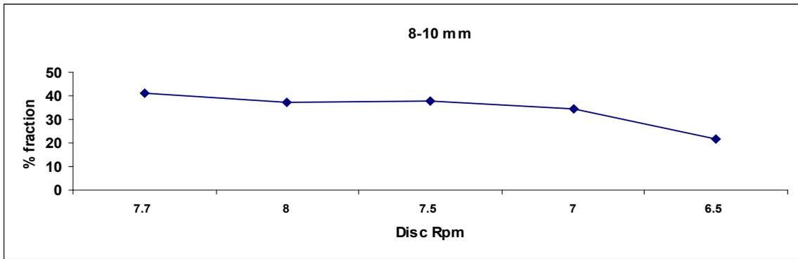
Figure 4. Fraction of 8-10mm size of green pellet vs. Disc rpm
