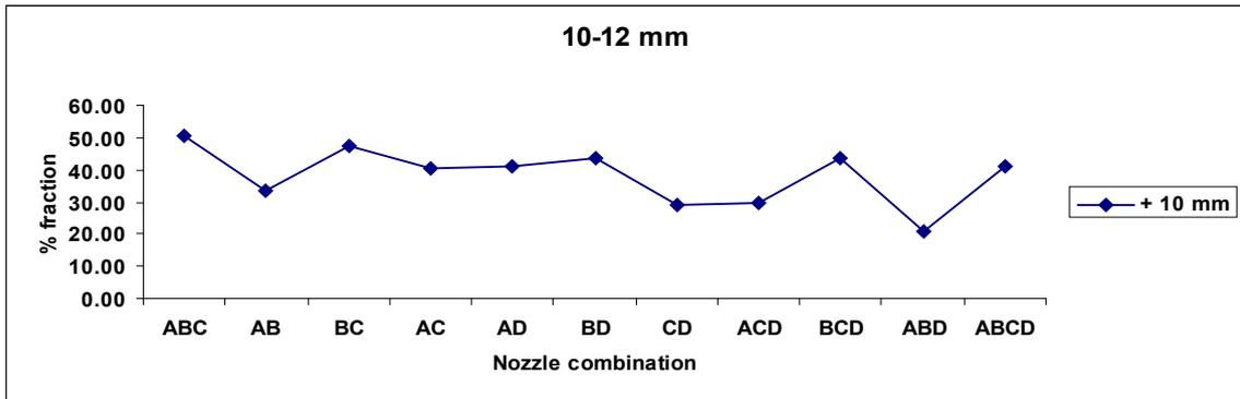
Figure 13. Fraction of 10-12 mm green pellet vs nozzle combination
