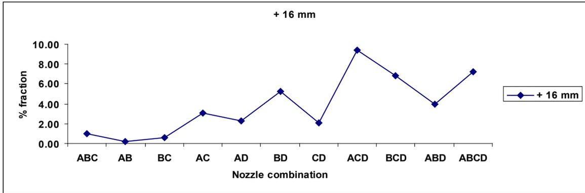
Figure 15. Fraction of +16 mm green pellet vs nozzle combination
