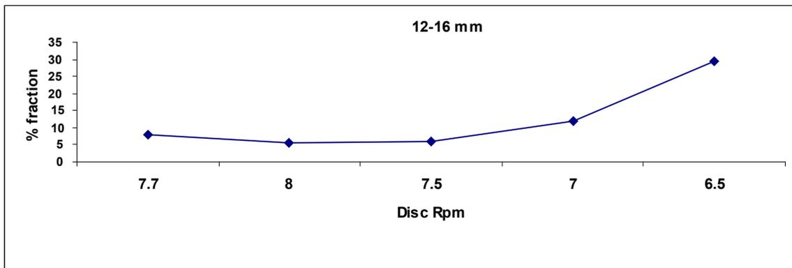
Figure 6. Fraction of 12-16mm size of green pellet vs Disc rpm
