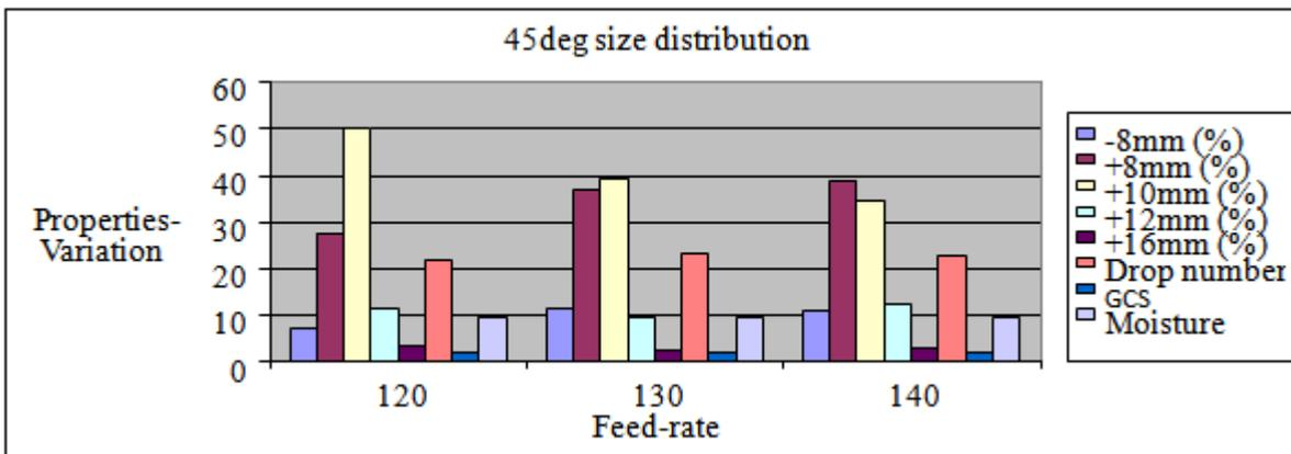
**Figure 21.** Properties variation vs. feed-rate (tph) at 45deg of disc inclination
