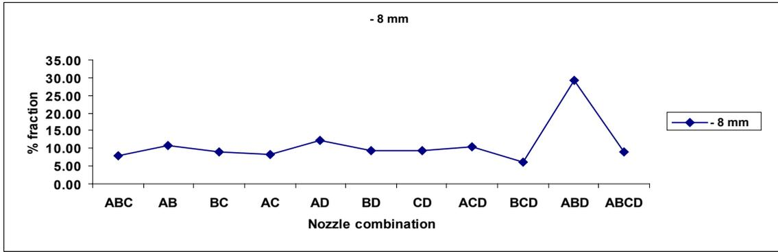
Figure 11. Fraction of - 8 mm green pellet vs nozzle combination
