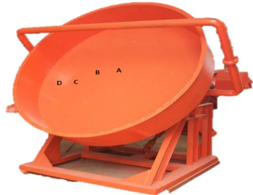
Figure 2. Balling disc with nozzle positions
