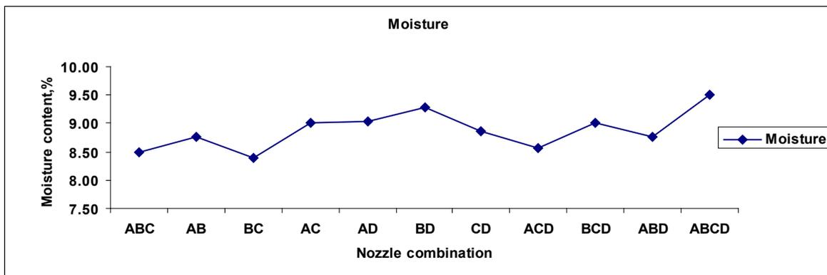
Figure 18. Moisture content vs nozzle combination
