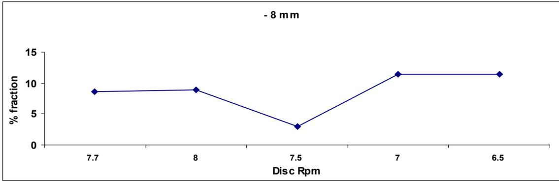
Figure 3. Fraction of -8mm size green pellet vs. Disc rpm
