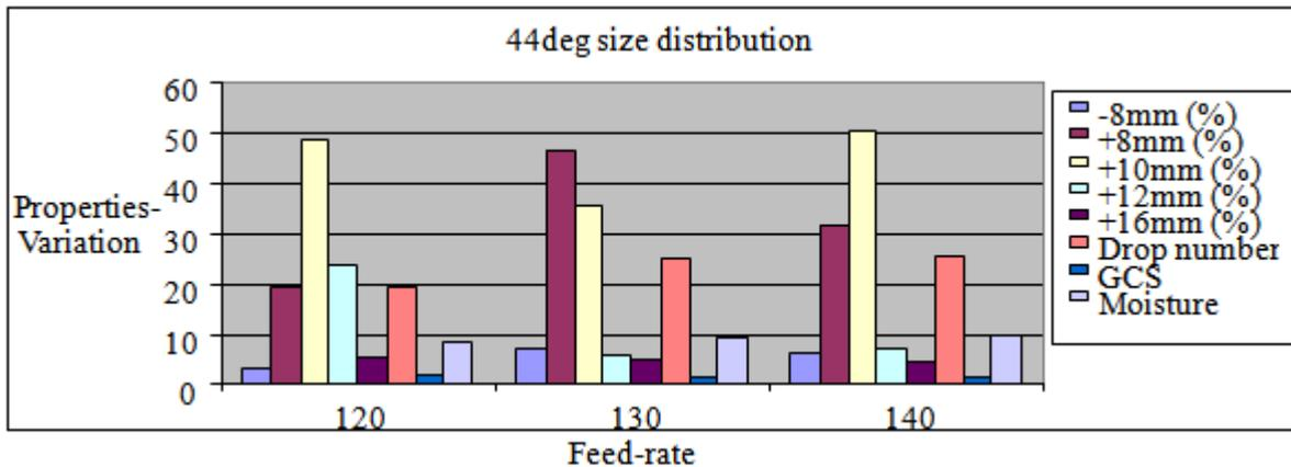
**Figure 20.** Properties variation vs feed-rate (tph) at 44deg of disc inclination
