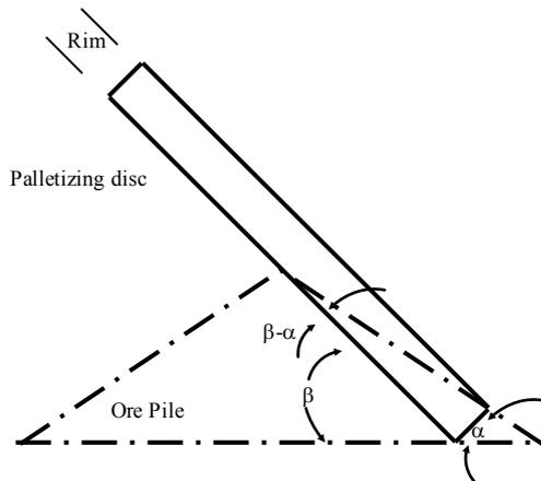
Figure 1. Orientation of Disc Pelletizer
