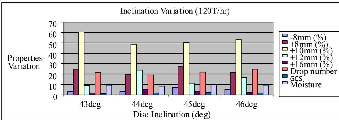
**Figure 23.** Properties variation vs. disc inclination at feed-rate of 120tph
