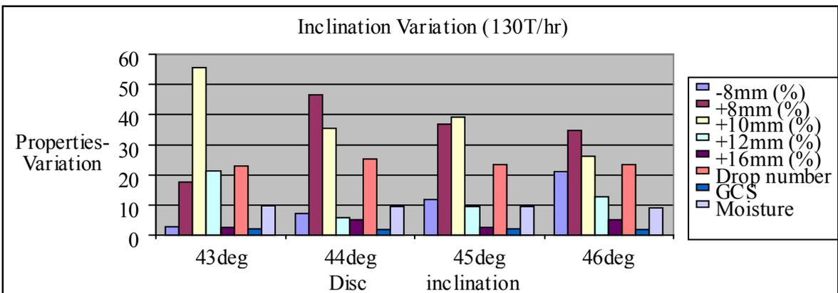
**Figure 24.** Properties variation vs. disc inclination at feed-rate of 130tph
