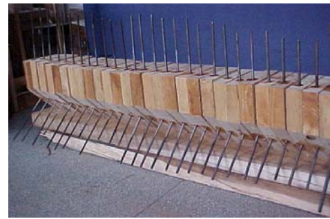
Figure 4. Pinus oocarpa Shiede specimens with glued steel bar
