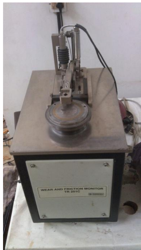
Figure 1. Pin on disc setup
